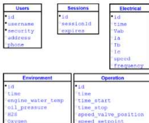
Fig. 3. Database schema in MongoDB at server side.
